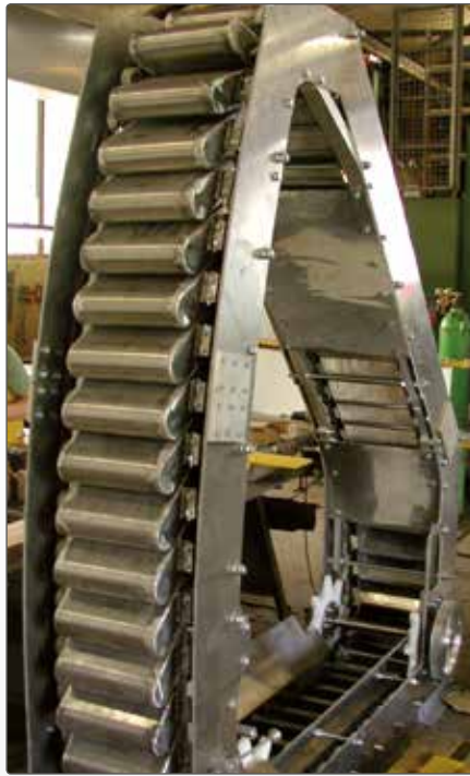
inner ejecting bucket elevator
