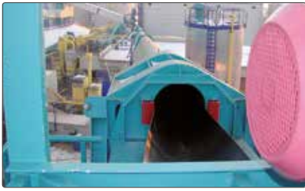
tubular belt conveyor
